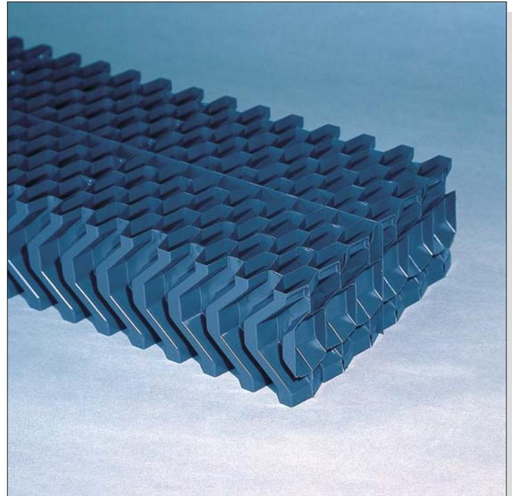
**THE DRIFT130 DRIFT ELIMINATOR**, with a geometry based upon 4 changes in the discharge airflow direction, is applied in situations of vertical airflow : it is constructed from preformed PVC sheets, subsequently made up into panels.
